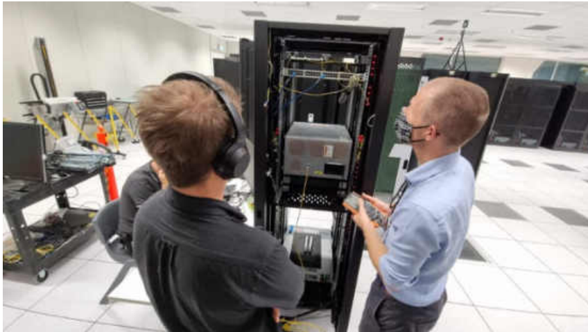
The world's first room-temperature, on-premises quantum computer in a supercomputing centre, designed, manufactured and deployed by Quantum Brilliance at the Pawsey Supercomputing Centre.
