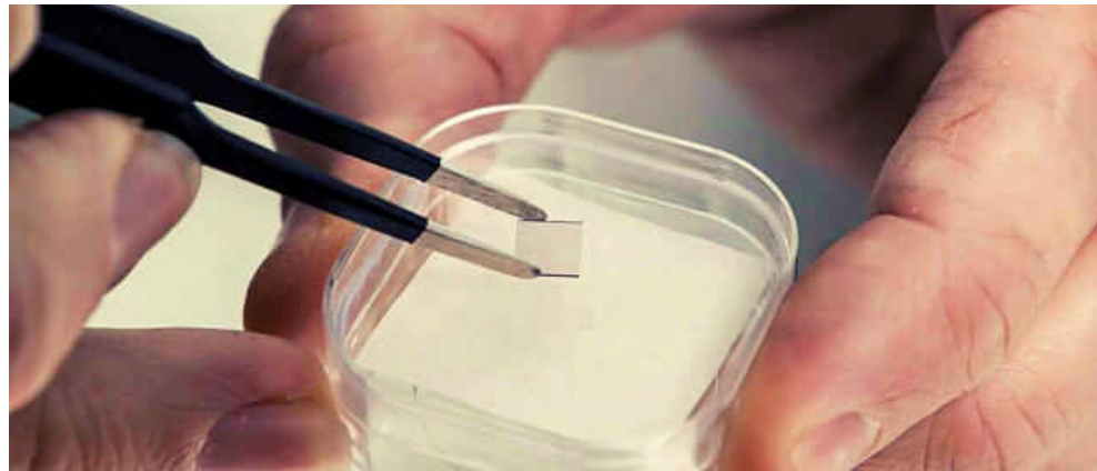
Top: Dr Marcus Doherty, Co-Founder and Chief Scientific Officer in the Quantum Brilliance Lab at the Australian National University. Bottom: a quantum-grade synthetic diamond used for room temperature quantum computing.
