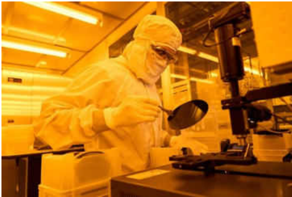
Rigetti employee inspecting a wafer of quantum chips at the company's Fab-1 facility in Fremont, CA
